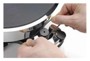
Now fit the lateral suspension O-rings to each suspension tower.
