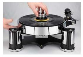
Holding the underside of the platter with your fingers, place the clamp onto the spindle. This gives you control of the platter whilst not leaving unsightly fingerprints on the platter wall.
